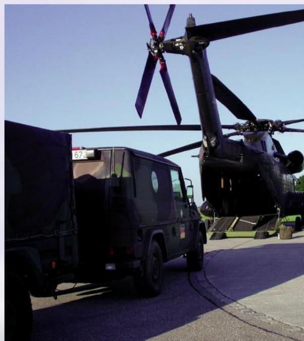
LUNA NG TUAS deployment by helicopter, using jeeps as Ground Control Station and transport vehicles
