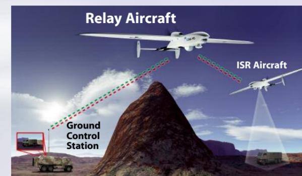
ISR with a relay payload – even in radio-shadow
